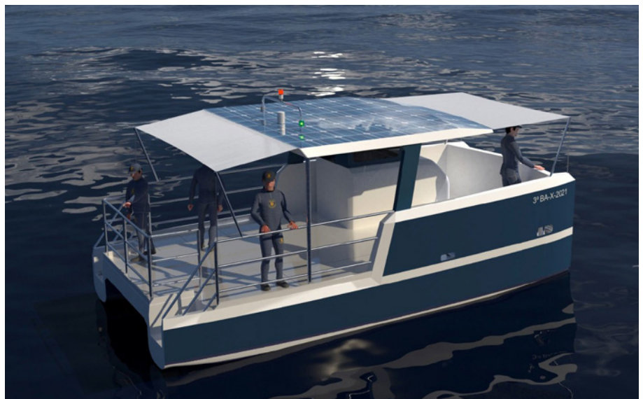
Figure 4: Design for solar-powered fishing catamaran (Source: Empordamar)
