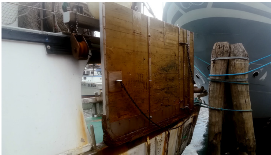
Figure 7: Otter boards with wood panels in use in the Chioggia otter trawl fleet, Italy (Source: DG MARE, July 2022, Sept. 2022)
