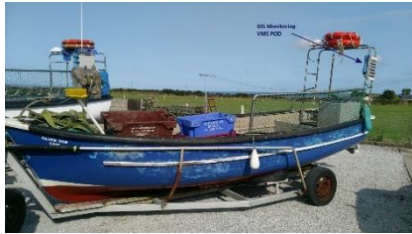
iVMS unit and gear sensors on fishing vessel
