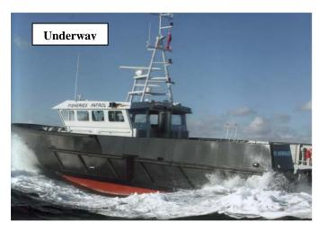
at 2,100 revs develop 520 kW each giving a top speed, on trials, of 13.5 knots. During normal patrols the engines are run at 1750 to 1800 revs allowing the vessel to cruise at an economical speed of approximately 11 knots. The St. Oswald also carries a 6 metre RIB which is stored in a stern ramp, making both launch and recovery safer and quicker. The system means that the RIB, is with the vessel
