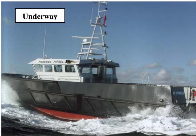
at 2,100 revs develop 520 kW each giving a top speed, on trials, of 13.5 knots. During normal patrols the engines are run at 1750 to 1800 revs allowing the vessel to cruise at an economical speed of approximately 11 knots. The St. Oswald also carries a 6 metre RIB which is stored in a stern ramp, making both launch and recovery safer and quicker. The system means that the RIB, is with the vessel
